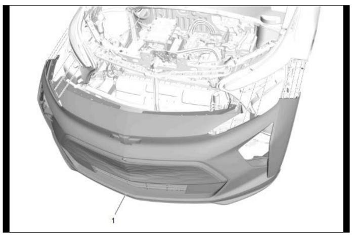
11. Reinstall the front fascia assembly (1). Refer to Front Bumper Fascia Removal and Installation in the Service Manual.
