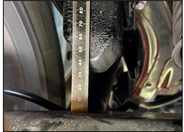
Figure 7. Bump Stop to Rear Axle Housing Gap
