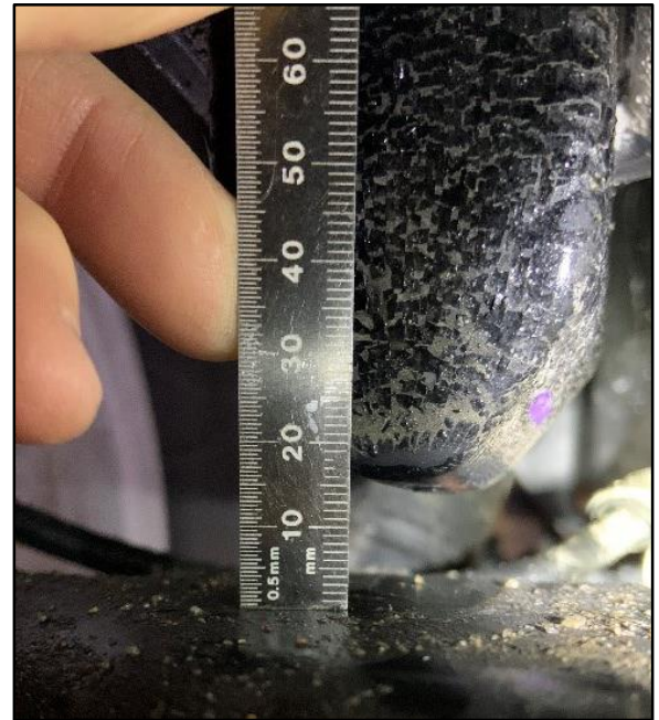
Figure 4. Bump Stop to Rear Axle Housing Gap
