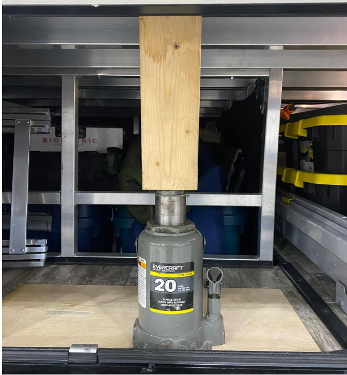
Photo example 2. Using jack to support rear upper deck.
