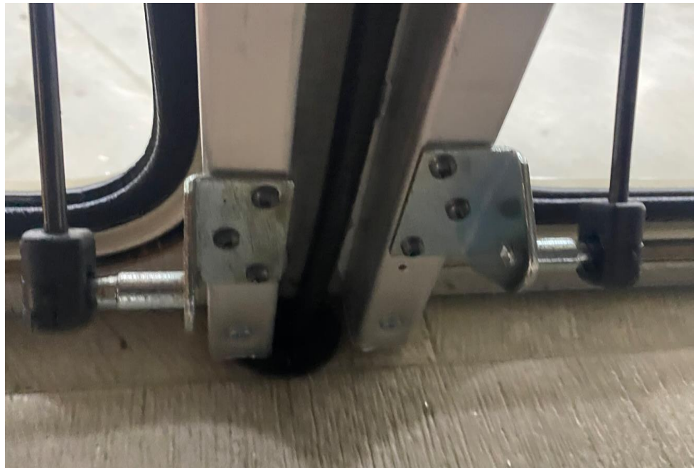
Photo example 6. Cargo door struts reattached.
