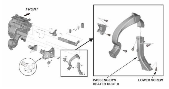
2. Push the passenger's heater duct B to give clearance for the blower motor to be removed and disconnect the motor connector.
