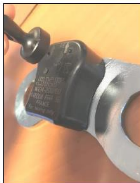
Figure 13: Use the magnet to change mode of WEM
