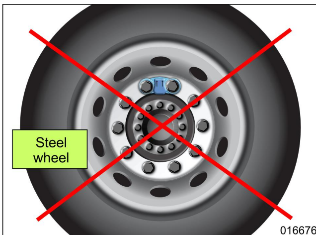
Figure 6: Installation on steel wheels is not allowed!
