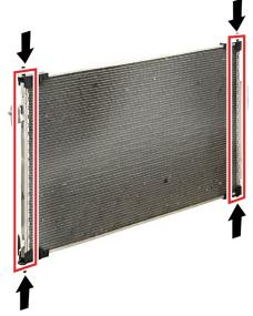
3. Check the inlet and outlet joints and the dryer cap for leaks.
