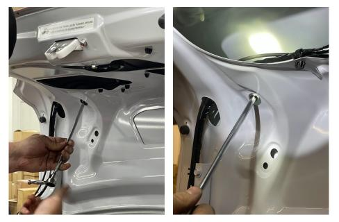
2. Insert tool between the Air Spoiler and trunk lid, then gently pry to remove.
