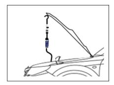
• **STEP 6:** Remove the purge hose and connect the hose from the applicator tool. Refer to the images below for the hose locations.
