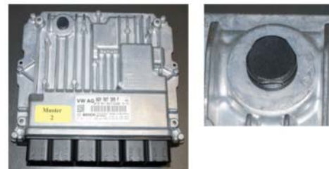
Pressure compensation element on DME control unit
