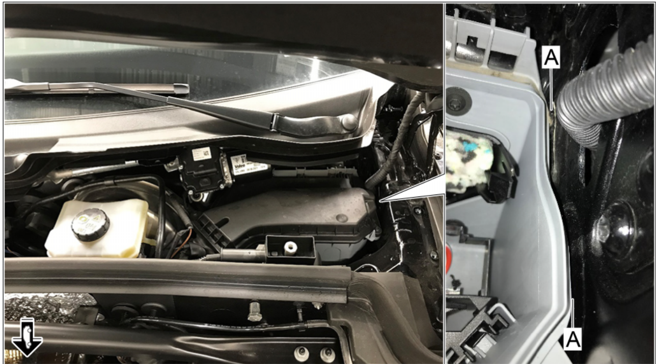
Gap from fuse box to unpainted bodyshell with PVC seam
