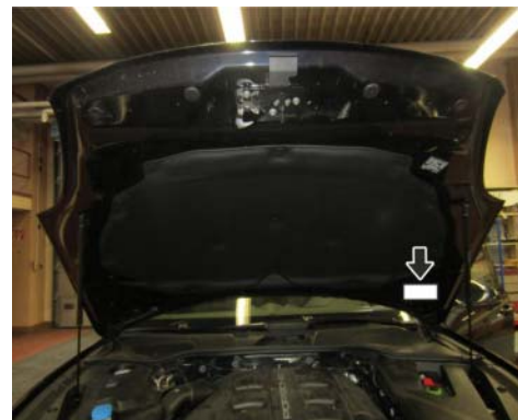
Proof of Completion Label: specified position (Exemplary illustration — 911 (991), Boxster/ Cayman (981) position accordingly)
