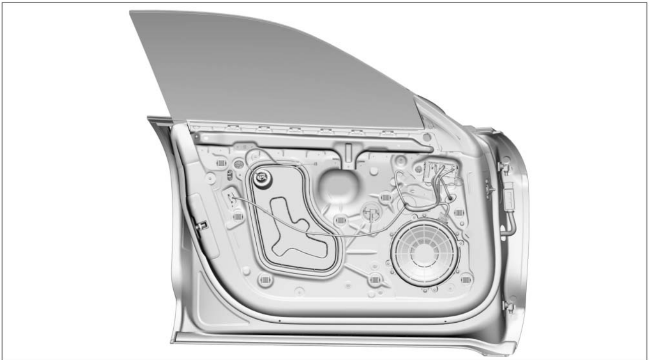
View of front door without door panel
