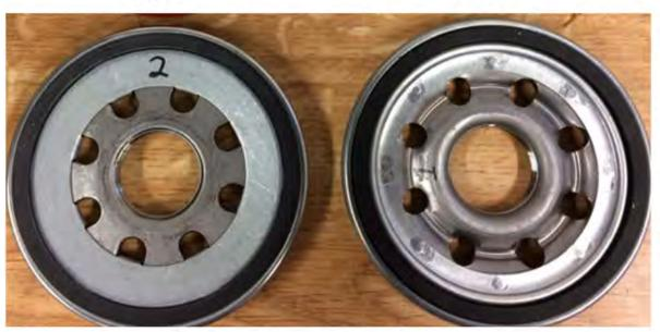
Volvo 21879886 Shallow Groovewill not fit on the US2017 fuel filter housing
