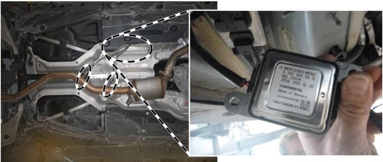
Figure 2 (example for model 166: NOx sensor and soot particulate sensor downstream of SCR catalyst)
