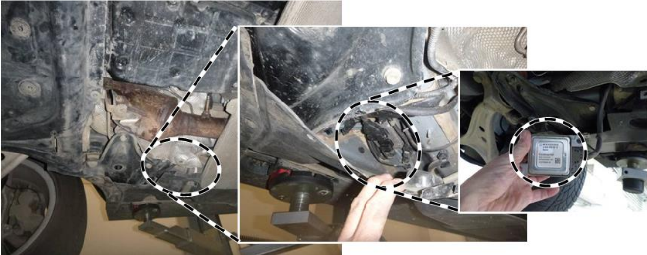
Figure 1 (example for model 166: NOx sensor upstream of SCR catalyst)
