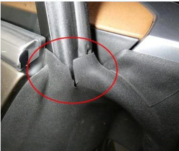
Figure 1 (Door seal split and division bar seal worn)
