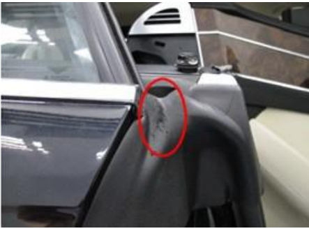
Figure 3 (Door seal worn)
