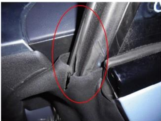
Figure 2 (Seal split and division bar seal worn )
