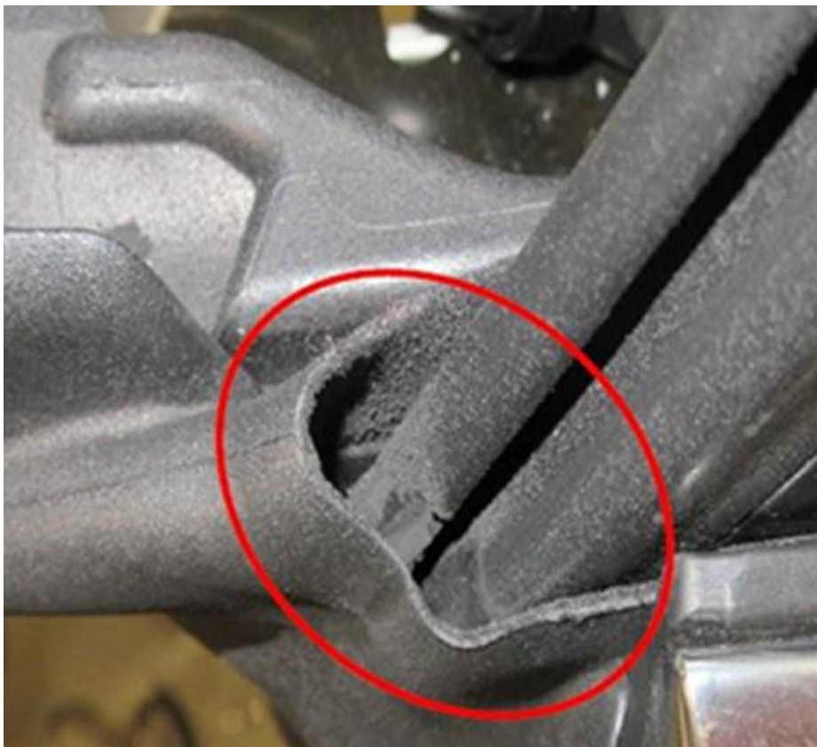
Figure 5 (Door seal worn and division bar seal worn/split)
