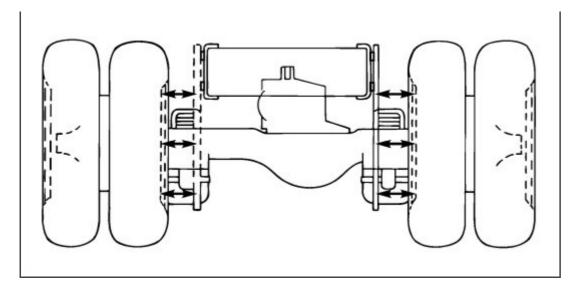
The maximum allowable difference between the measurements taken at the front-rear and rear-rear brake drums to the straightedge must not exceed 6.4 mm (1/4 inch), whether or not the chassis is equipped with a transverse torque rod
