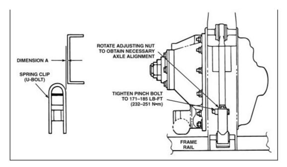
To obtain proper axle positioning, adjust the adjustable transverse torque rod as follows:
