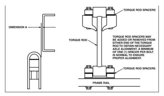
4. After axle centring is verified or corrected, exhaust the air from the suspension and verify that no interference exists between the frame rail and any spring clip (U-bolt).
