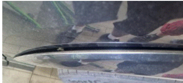
Figure 2. The front wheel arch trim with the retaining clips only partially engaged.
