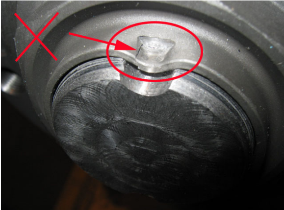
FIGURE 14: BROKEN OR TORN LIP – REJECTED
