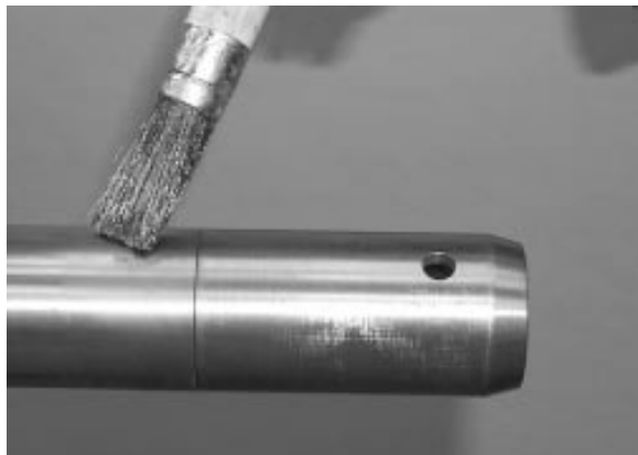
FIGURE 32: APPLY GLEITMO 805 GREASE
