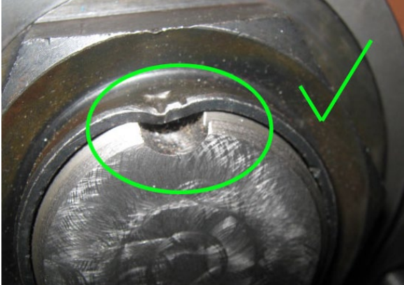
FIGURE 12: CORRECT - PREVENTS THE NUT FROM GETTING LOOSE
