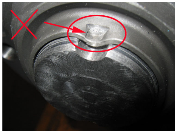
FIGURE 39: BROKEN OR TORN LIP – REJECTED
