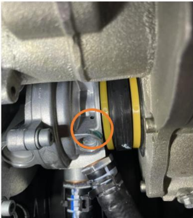
Figure 1.1 – Leak From Coolant Pump Expansion Chamber
