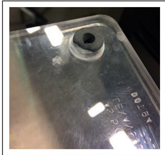
Figure 4 - Installation of New grommet on the Lexan Panel
