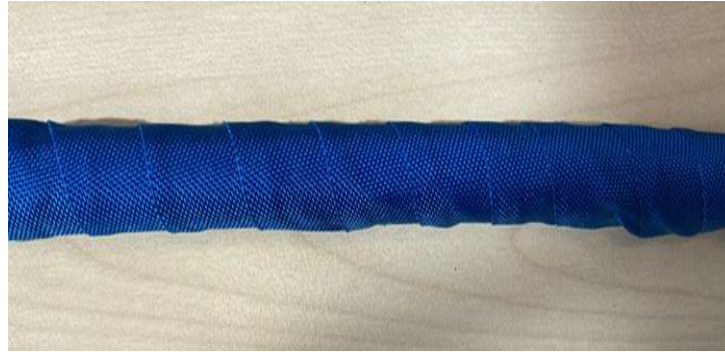
Figure 6: Cable wrapping for N 107 292 04 (blue).
