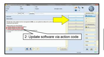
Select the correct option to "Update software via action code" OR "Software update via measured code".
