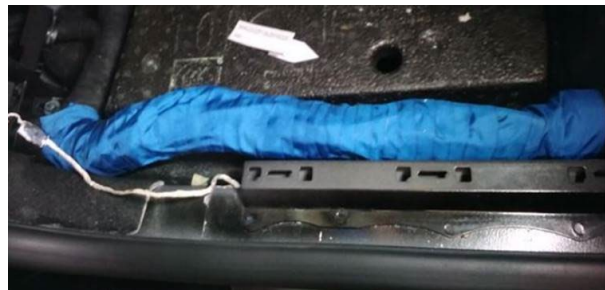
Figure 10: Main wiring harness wrapped with blue textile tape.
