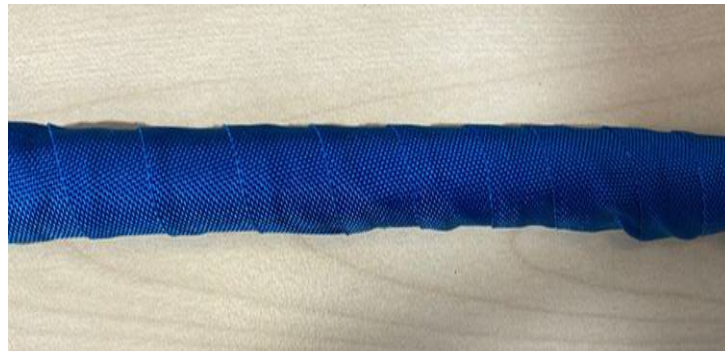
Figure 6: Cable wrapping for N 107 292 04 (blue).
