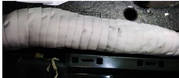
Figure 11: Gray textile tape covering the already wrapped main wiring harness.
