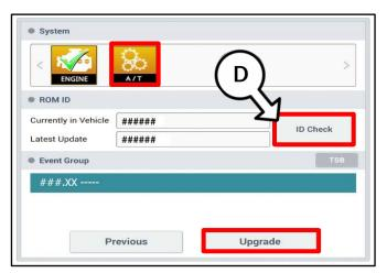
The ECU upgrade will begin and the progress of the upgrade will appear on the bar graph. Upgrade part (1/2) (E) will download the upgrade event to the VCI-II. Upgrade part (2/2) (F) will upgrade the ECU.
