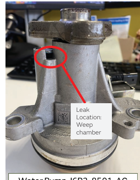
Water Pump J6P3-8501-AC LR Service Number: LR121418 Jaguar Service number: T4A41037
