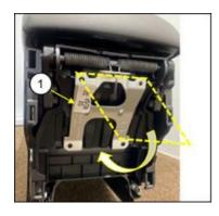
11. Tighten the screw from the upper right side (1), then remove the jig.
