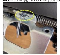
10. Push the bracket down to the position (1) as follows.
