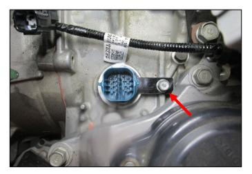
20. Remove the ATF warmer, located on the valve body cover.
