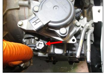
33. Reconnect the 12V safety plug located on the passenger side of the engine bay.
