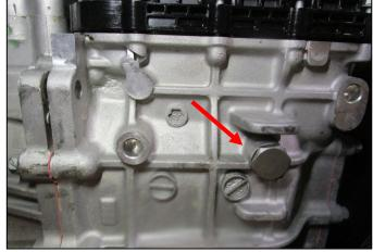
14. Remove the hybrid cooling system drain plug and drain the coolant.
