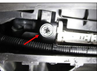
15. Disconnect the TCU connector and remove the TCU.
