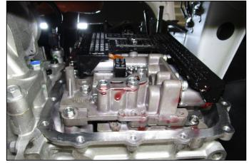
30. Install a new valve body cover gasket. P/N 45283-3D100.
