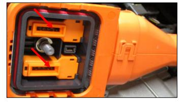
10. Measure the voltage between the power cable(+) terminal and chassis ground.
