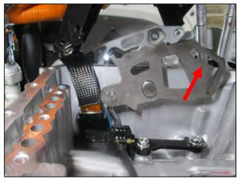
28. Confirm the manual shaft is inserted in the slot in manual lever.
