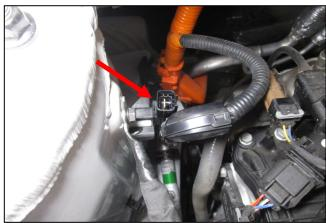
34. Reconnect the high voltage plug, located on the driver's side near the radiator.
