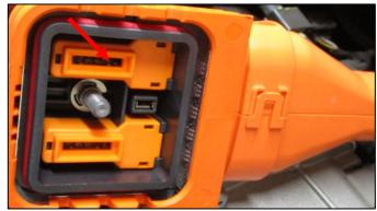
11. Measure the voltage between the power cable (-) terminal and chassis ground.
