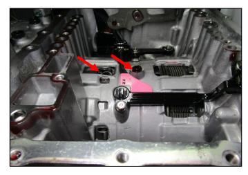
27. Move the harness up and out of the way so the valve body can be reinstalled.
