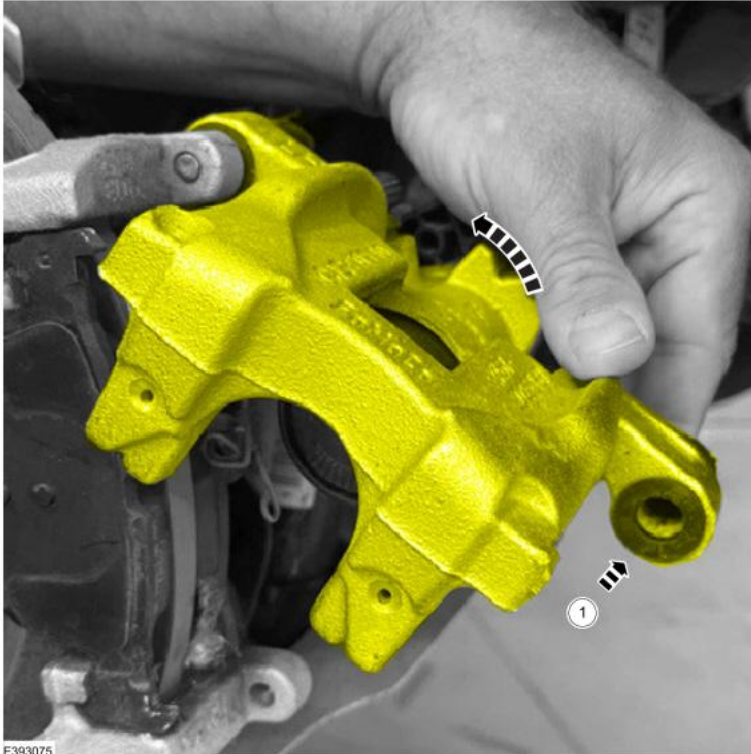
7. Using 6 in. slip joint pliers, remove and discard the standard bushing located on the opposite side of the bleeder. (Figure 7) Figure 7
