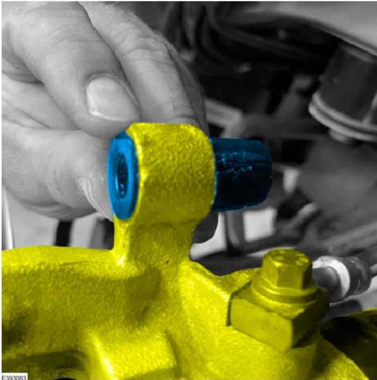
9. Rotate the rear caliper downwards. (Figure 15)
