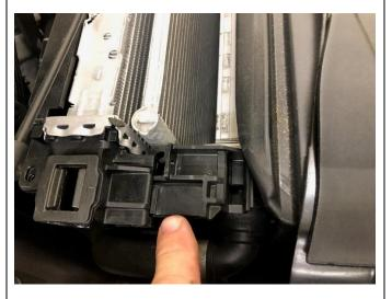
11. There are plastic push tabs that must be depressed to release the AC condenser from the cooling module. This is on the passenger's side.
