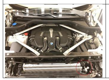
10. There are plastic push tabs that must be depressed to release the AC condenser from the cooling module. This is on the driver's side.
