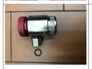
13. Only the R134a adapters fit the quick disconnects of the AC machine.
