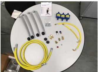
12. The flush machine (Robinair or Mahle manufactured) will come with hoses, filter, and hardware. Pictures are of the Mahle flush kit as received.
