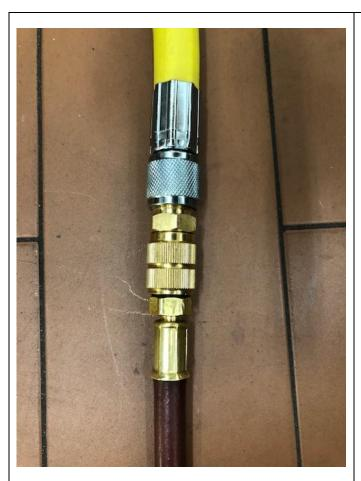
15. **Y1234a high side adapter installed** in place of the quick disconnect
