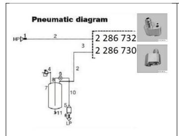
1 HP outlet adapter fitting High-flow connection hoses 2 3 Item to be flushed 4 Safety valve 18 bar / 261 psi 5 Filter15 µm LP fitting 6 7 6 liter fluid vessel Connection hose between vessel and 8 sight glass 9 Fluid indicator sight glass with cap 10 Connection hose between sight glass and filter 11 Auxiliary valve with cap
