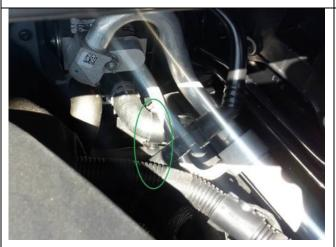
Mount a spacer (part number 11 53 7 537 923) in the engine compartment between the coolant hose feed and coolant hose return.
