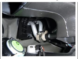
Tape the two heat exchanger lines with a felt strip (part number: 51 45 2 353 024) 4-5 inches (10-12 cm) long around each of the lines. Secure the lines together using a worm-type hose clamp (part number 07 12 9 952 117).
