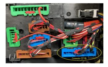
2. Locate and disconnect the blue connector (**Z2\*1B)** from rear power distribution box.
