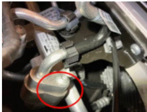
Figure 11. Service port mounting interference with adjacent line.
