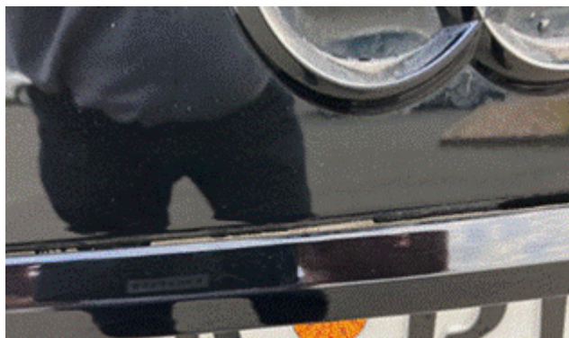
Figure 1. Tail lamp trim molding loosening.
