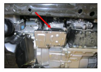
7. Disconnect the harness connector from the transmission
