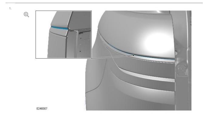
Inspect the outer tail lamp and rear quarter panel gap on both sides of the vehicle.
