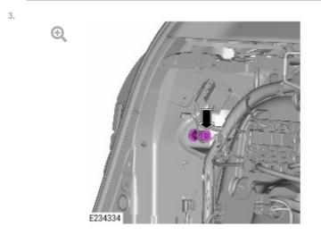
Remove the outer tail lamp fastener.
