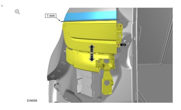
Adjust the outer tail lamp so there is a 1 mm gap between the outer tail lamp and the rear quarter panel.
