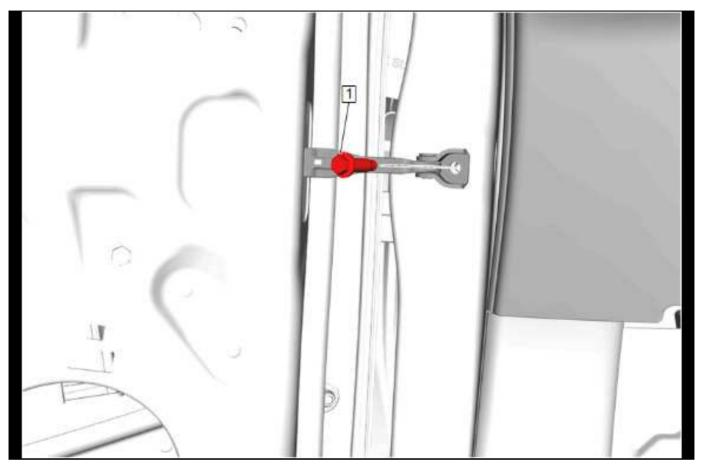
2. Remove the bolt (1) that secures the doors check strap to the A-pillar.
