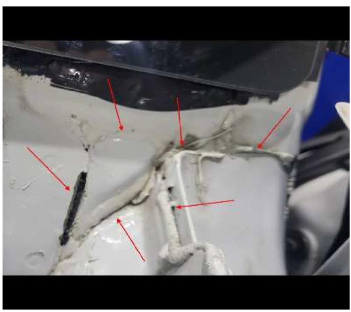
15. Locate the seams where the A-pillar merge to the plenum panel and inner fender as indicated in the graphic above.
