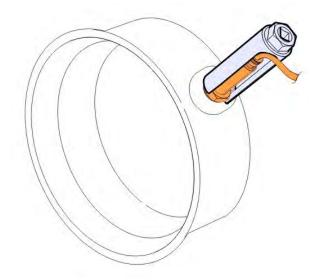
• If damage to the threads occurs when removing the sensor, replace the bung as outlined in Technical Servic Fittings, One Box, Replacement. PM, NOx and Temperature Sensor Fittings, found under the service tab in Imp
