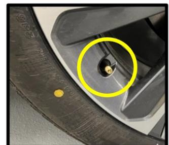
**NOTE:** If some transmitters are not activating, attempt to repeat the process after rotating the affected tire(s) 90 to 270 degrees.
