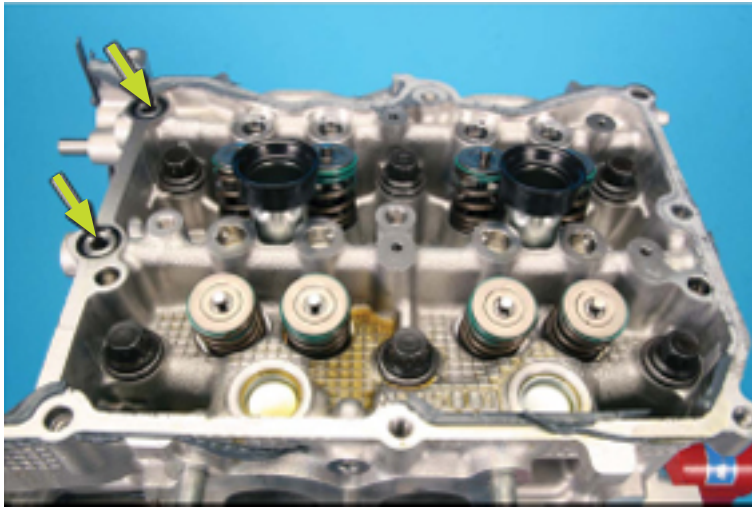
Cam carrier o-rings requiring replacement
