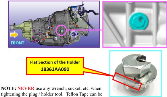
tightening the plug / holder tool. Teflon Tape can be applied to the holder threads for added stability.
