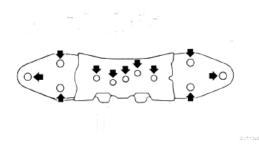
• Lower the transmission stand by **NO MORE THAN 75mm**. Remove the 6 bolts securing the transmission cover then CAREFULLY slide cover toward the rear of the vehicle.
