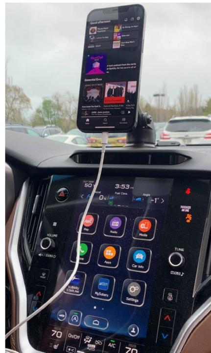
Finally, with the addition of CP1 to the Subaru lineup, there is a much larger screen where multiple inputs can be made. Shown to the right is an example of how a charging cord could affect the screen. This is especially noticeable in radio mode or a screen with several selections such as SXM or Navigation. This could cause a no response situation or screen distortion until the key is cycled and the cord is removed.
