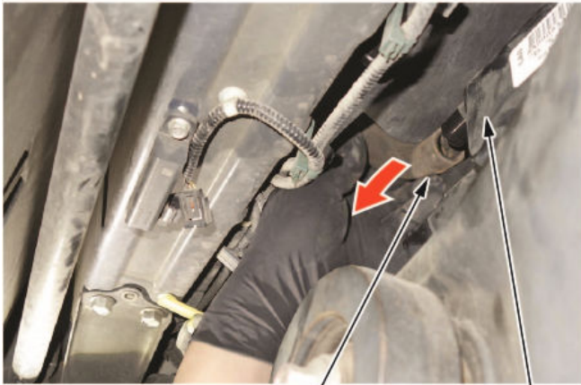
Disconnect the rubber drain tube. EVAP CANISTER
