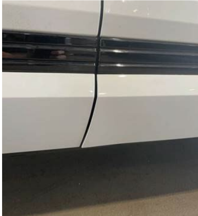
Figure 1. Door cover trim as it appears when loose.
