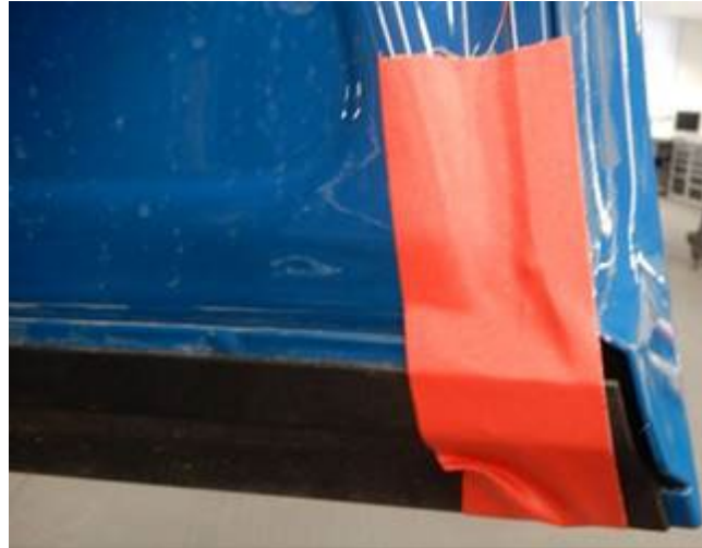
Figure 7. Painter's tape binding the newly adhered trim pieces.
