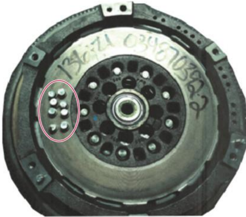
Figure 3 - Stuck dual mass flywheel due to spring breakage. Bolt access requires cutting through the flywheel.
