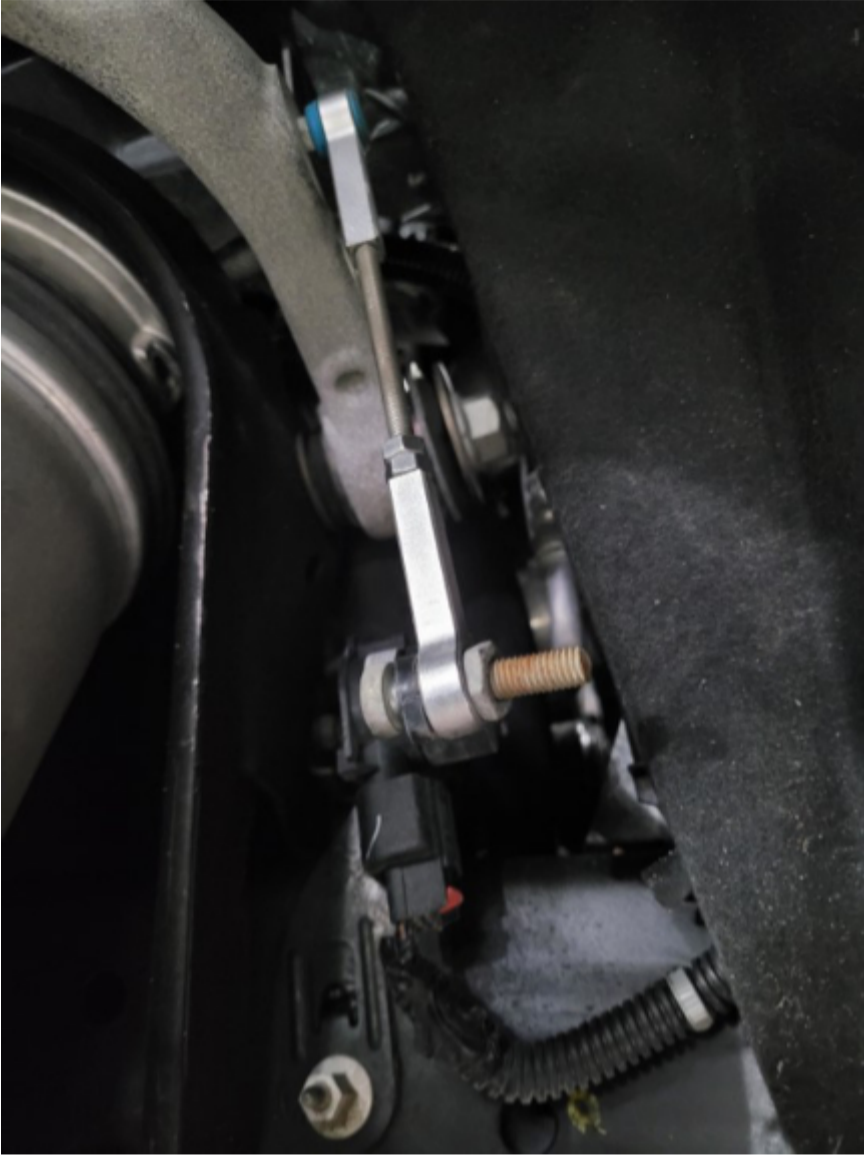
Notice Angle or Rear Axle Drive Shaft due to suspension being lowered.
