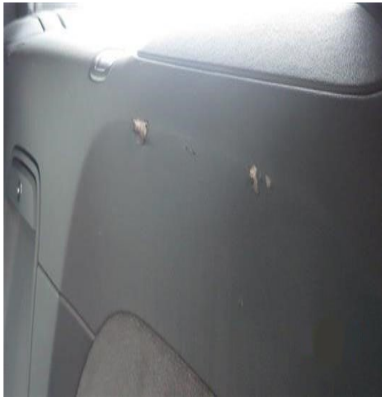
Figure 1. Damaged rear panel trim panel.
