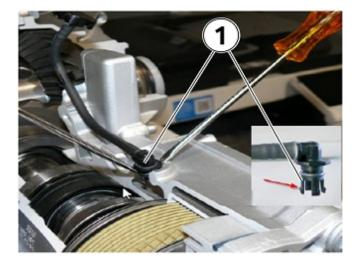
Carefully pinch the tabs on the old vent line and pry it out of the housing (1).
