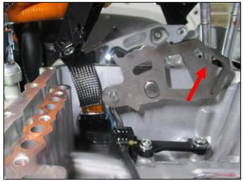
31. Confirm the manual shaft is inserted in the slot in manual lever.
