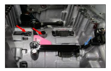
30. Move the harness up and out of the way so the valve body can be reinstalled.
