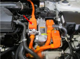
8. Wait more than <u>3 minutes</u> so the capacitor in the high voltage system can be discharged.
