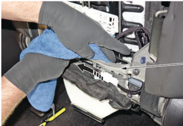
METAL SEAT FRAME Clean the inside surface.
